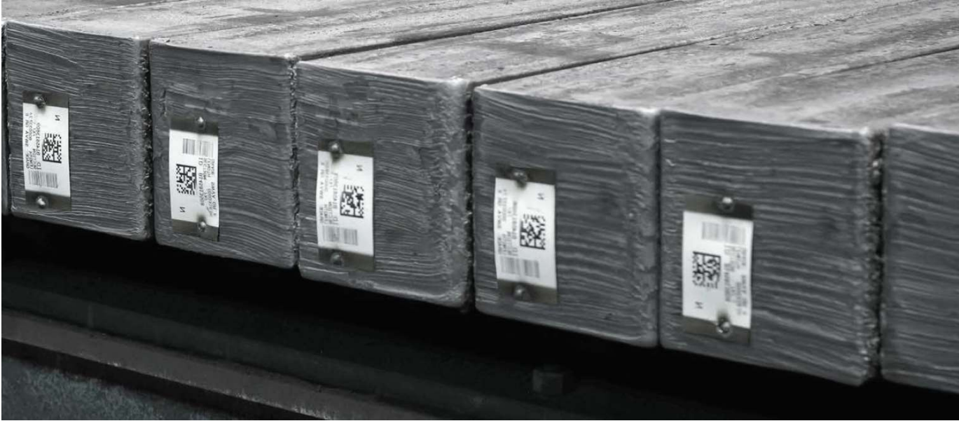
Continuous cast semi-finished billets, capable of producing to a wide range of chemistries and test requirements, please inquire.
