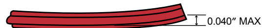
Top view of rail lateral (horizontal) line of tolerance at rail ends.
